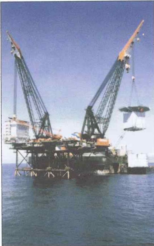
The giant semisubmersible crane vessels – Balder (left) and Hermod (right) – in their North Sea prime. Balder is pictured installing two modules simultaneously on the Ninian Northern platform, 1979.
